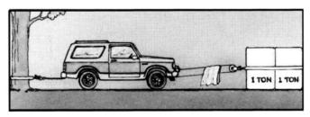
To double the pull, use 2-part line and tie off to chassis. Take out of gear.
