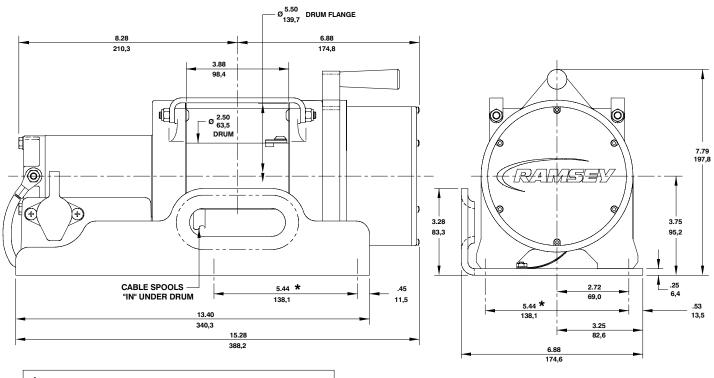
\*MOUNTING BOLT PATTERN: FOUR Ø.406 HOLES IN A 5.437±.015 x 5.437±.015 (138,1mm x 138,1mm) RECTANGULAR PATTERN.
