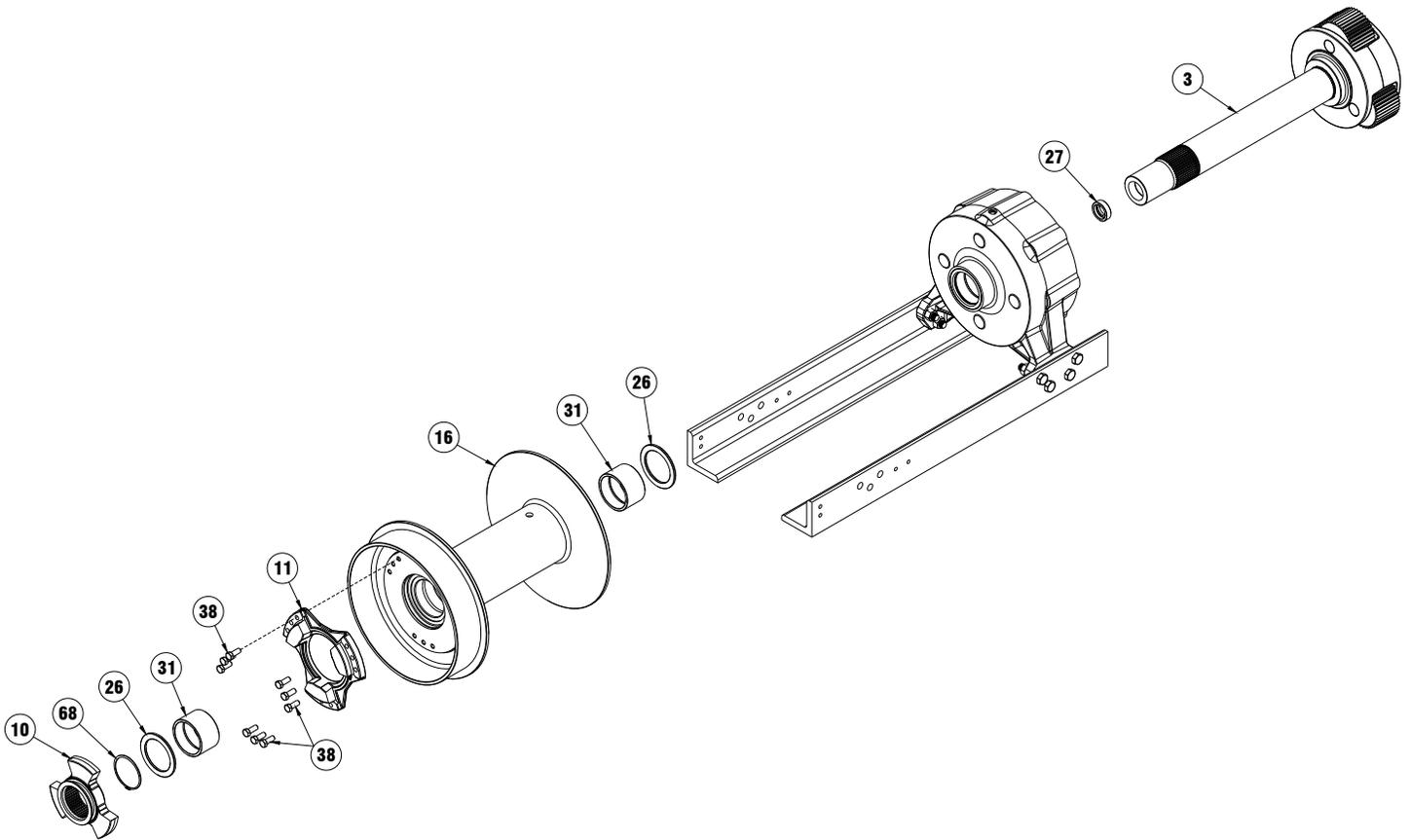
27. To remove gear end bearing #21, from mounting angles #7 and #8, first remove (4) bolts #40 and (4) nuts #42 from each angle. Shaft oil seal #66 and end bearing bushing # 31 can be removed and replaced at this time, if necessary.
