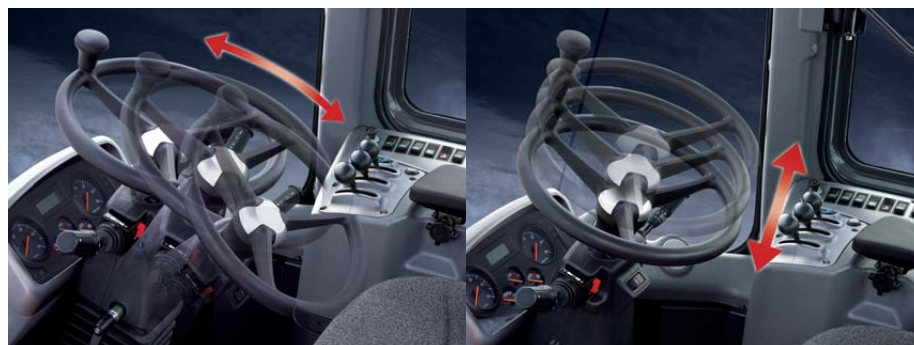
The steering Column The steering column features both tilting and telescopic functions.
