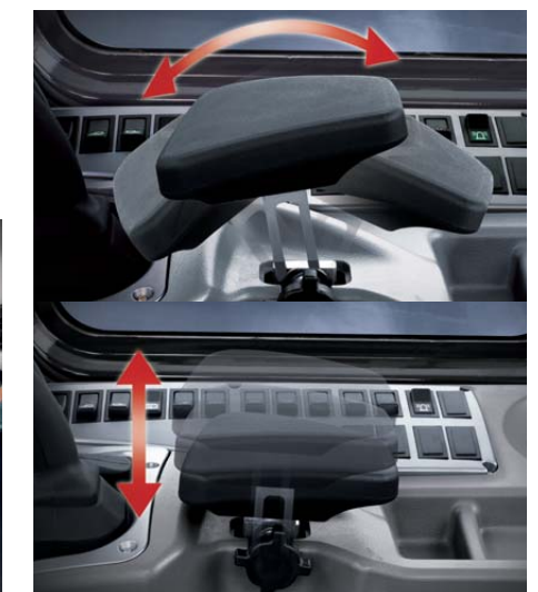
Wrist rest The tilting and telescopic wrist rest allows the operator to work more comfortably.
