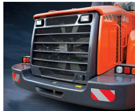
Radiator Grill (Steel structure)
