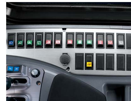
Switch The ergonomically laid out switch panel in line with the natural movements of the body allows for very convenient operation. The spare switch cut-outs allows easy installation of additional electric accessories.
