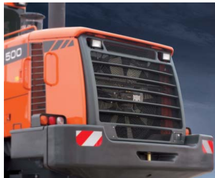
Radiator Grill (Steel structure)
