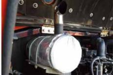
**Double Noise Absorber** New noise absorber further lowers noise level. Engine room overheating is prevented to improve work comfort and machine durability.
