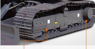
The track roller attachment point was shifted from lower to middle portion to improve undercarriage stability and structural rigidity of the chassis.
