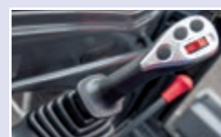
Proportional joystick with auxiliary thumb control
