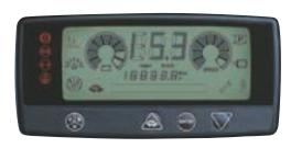
The combination of LED displays and 7-digit graphic LCD display intelligently provides operators with all the information they need, including operational information, diagnostics, and programmable settings. The 4 display buttons offers a choice of four power modes; heavy duty, standard duty, economic duty and slow travel speed mode. Standard instrument images are displayed at the right.
