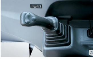
The hydraulic joystick levers have very comfortable grips and allow the operator to perform precise operations very easily. As there are 3 switches on each lever, attachment can be easily operated.
