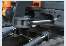
The convenient boom swing function provides the ability to work in very narrow locations, and the robustly designed swing bracket and large boom swing cylinder ensures powerful and stable boom swing performance.
