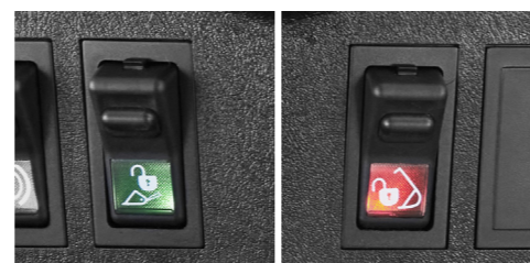
Safety Switch (Loader)
